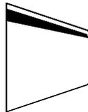
The TRUNCATED CONICAL or TC style is a cut-off (truncated) cone shape. It can be made without a shoulder, in the TC point form die.
