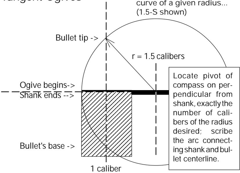
Locate pivot of compass on perpendicular from shank, exactly the number of calibers of the radius desired; scribe the arc connecting shank and bullet centerline.
