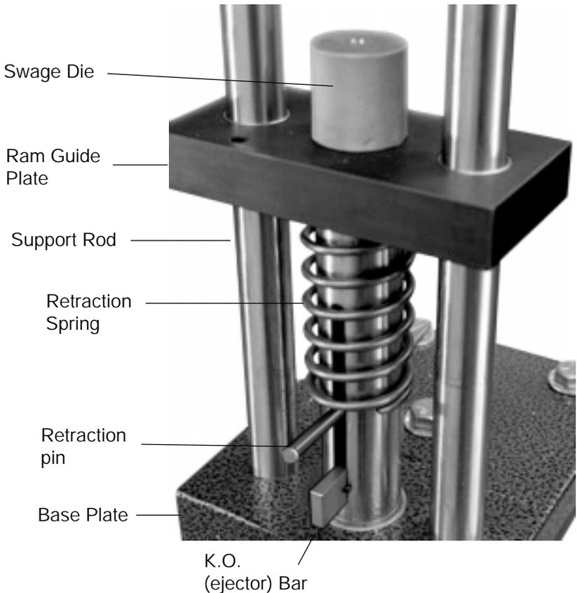
The Retraction Pin fits through a hole in the internal punch head for those punches which require it, beneath the last coil of the Retraction Spring. The ram must be raised to insert the pin.
