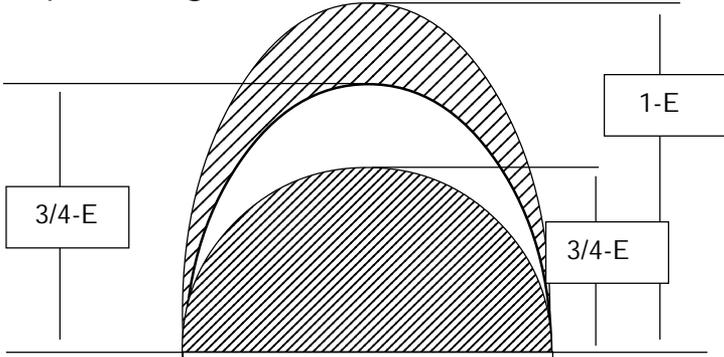
Common elliptical ogive shapes (.5-E is the same as .5-S, a half-ball). Elliptical ogives are measured along the bullet centerline axis from start of ogive to the tip. The ogive is half an ellipse.
