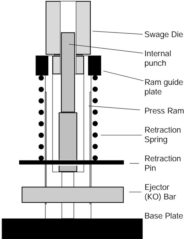
Several heights of KO Bars are provided with the Mega-Mite press to use with different lengths of dies and punches. Because the stroke length of the Hydro-press and Hydro Junior is adjustable, only one height of KO Bar is required for all lengths of dies and internal punches.
