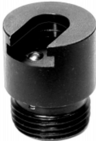
The Corbin RLA-H reloading shell holder adapter features a spring-loaded ball bearing detent to smoothly hold standard RCBS type shell holder buttons securely and yet allow them to be easily replaced. The T-slot fits current RCBS brand shell holders: other brands or earlier versions having different tolerances or dimensions may not fit without modification.
