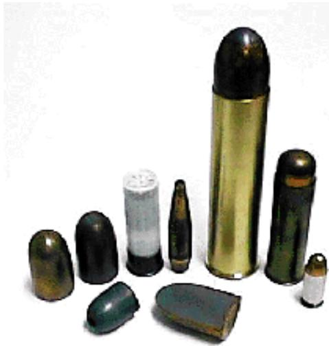
2. Left to right in rear: 22mm jacketed projectiles, one solid, one soft point, 12-gauge shotgun shell for comparison, 50 BMG Ultra Low Drag RBT design with open tip, 4-Bore loaded cartridge, 10-Bore loaded cartridge, .45 ACP for comparison.
