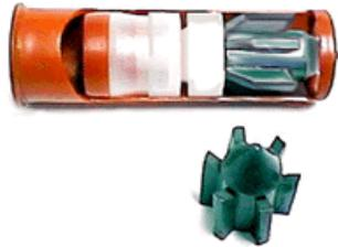
1. Delta-wing slug in 12 gauge, hollow base design, high velocity. Does not carry a payload.
