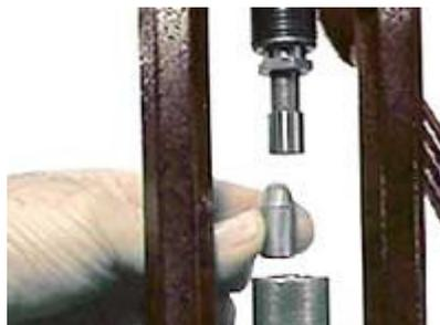
lower the ram. If the bullet comes out with the punch, adjust the die a little lower and swage again. When the bullet stays within the die, it has been expanded to the die bore size and is gripping the die walls. A thin film of swage lube is squeezed between the lead and the die surface, protecting the die.
