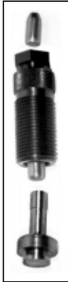
Bullets can usually be reduced 0.006 inches depending on the material strength and thickness of the jacket walls. It is possible to reduce .357 pistol bullets to make .355 (9mm) or to reduce a .323 rifle bullet to .318.
