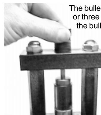
The bullets may not emerge until you have drawn two or three of them. With some diameters and lengths, the bullet can pop out with a sudden rush, perhaps flying out the top of the die with some force. Therefore, do NOT look down into the die or place any part of your face near the top of the die while drawing.
