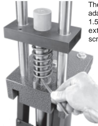
The CSP-2 comes with a reloading adapter kit, consisting of a 7/8-14 to 1.5-12 thread adapter bushing, a ram extension with primer port, and a screw-in T-slot shell holder adapter.
