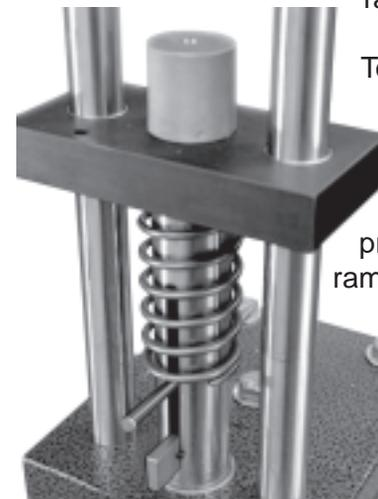
To install the pin, the ram is raised part way and the spring pushed up with the pin so it can be inserted through the punch head. The knock-out bar and the retraction pin should both project equally on both sides of the ram.
