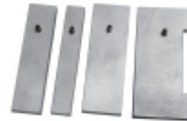
For bullet swaging, the die screws directly into the ram. A set of four knock-out bars is provided for use with different lengths of swage dies and punch heads. The hardened KO bar goes through the ram, below the internal punch. Use the KO bar that allows the punch to eject the bullet at the bottom of the stroke.
