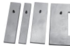
For bullet swaging, the die screws directly into the ram. A set of four knock-out bars is provided for use with different lengths of swage dies and punch heads. The hardened KO bar goes through the ram, below the internal punch. Use the KO bar that allows the punch to eject the bullet at the bottom of the stroke.
