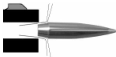
The RBT improves performance by deflecting muzzle gas instead of channeling it to the front of the bullet in a ball, as with conventional boattails. This can give up to 15% less dispersion at the target.
