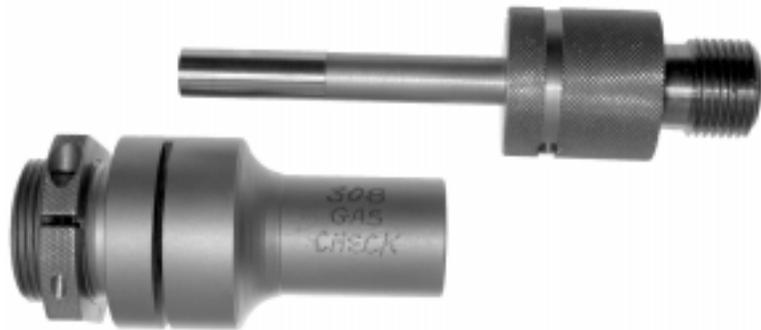
This die and punch set is used in the Corbin CSP-2 and CHP-1 presses to punch a strip of copper tubing, normally 1-in wide by .030-in thick, into proper diameter disks which are then used to make gas checks.
