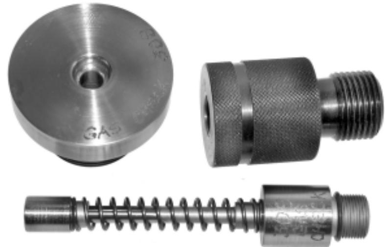
This die and punch set is used to draw a proper size disk of copper into a gas check. The die fits into the press head from the bottom, just the opposite of most dies. The large disk section faces the ram.
