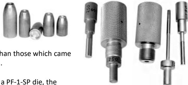
The maximum insertion line on another external punch of the same caliber may or may not be right for that particular die. This is because the die cavities, while held to close tolerance in depth, are hand lapped and will change depth slightly as the die is finished with diamond lap to the final stage of polish. The punches are precisely fitted to four decimal places by individually making slugs and testing, measuring and carefully cutting the punch to obtain a perfect match.
