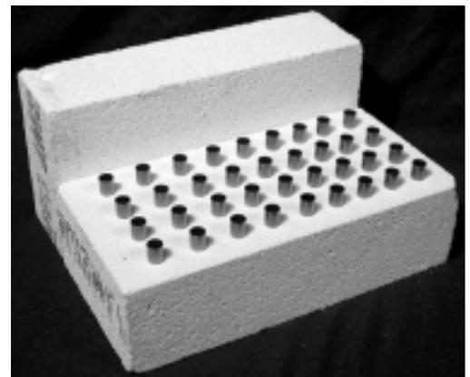
Cut out the above template and tape it to a ceramic block, with the edges carefully aligned. Poke a centering hole through each circle, through the template and into the block, to establish a drill pattern.
