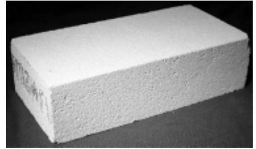
Ceramic block is 9 inches long, 4-1/2 inches wide, and 2-1/2 inches high. Cut out the actual size template (left) and tape it over a block. Use a scribe or other sharp steel object to make a small hole in the block at each of the cross-lines, in the center of the circles. Then remove the template...
