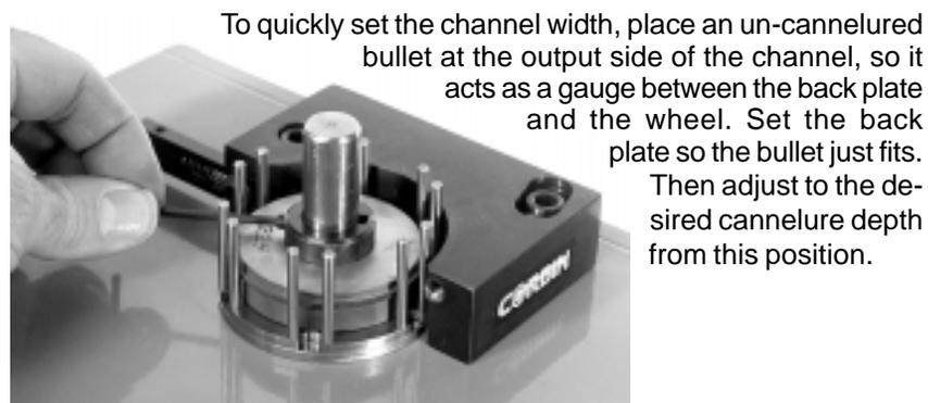
To quickly set the channel width, place an un-cannelured bullet at the output side of the channel, so it acts as a gauge between the back plate and the wheel. Set the back plate so the bullet just fits. Then adjust to the desired cannelure depth from this position.
