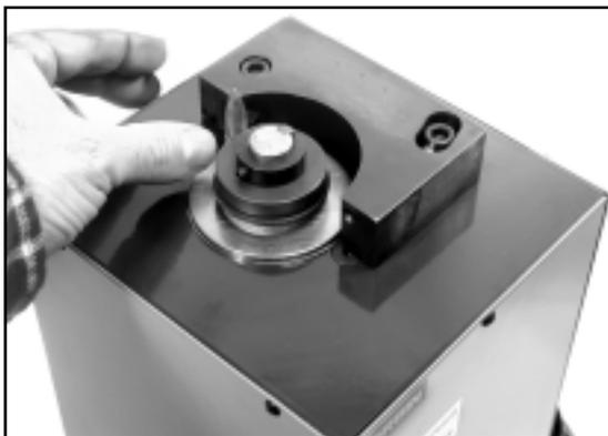
Standard cannellure width is .050-inches with a vertical serration. The raised portion of the wheel, which impresses the cannellure, is offset from the center of the wheel, so you can turn the wheel over providing different cannellure positions, in addition
