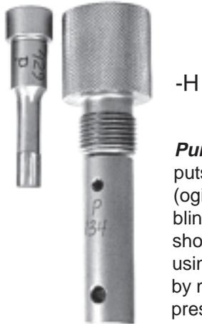
**Purpose:** The point forming die puts a smoothly curved nose (ogive) on the bullet. The semi-blind hole eliminates the step or shoulder that would be created by using a punch. The bullet is ejected by means of a spring wire punch pressing against the very tip of the bullet.
