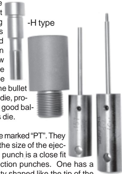
**Identification:** The die and punches are marked "PT". They are also marked with the caliber and the size of the ejection pin. The diameter of the external punch is a close fit to the die cavity. There are two ejection punches. One has a reduced solid tip, and one has a cavity shaped like the tip of the metal insert. This die can be added to any set and used instead of the standard point forming die, to make metal tip bullets.
