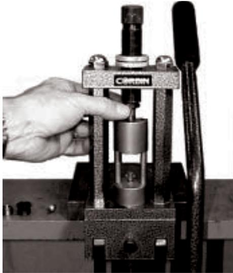
Installing the ball-forming die in the Corbin Series II Swage Press.
