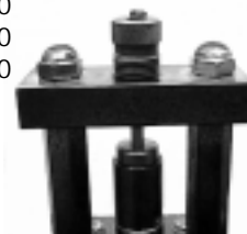
Bullet reducing dies work best when reduction is kept under .006 inches. Example: .323 to .318, or .357 to .351
