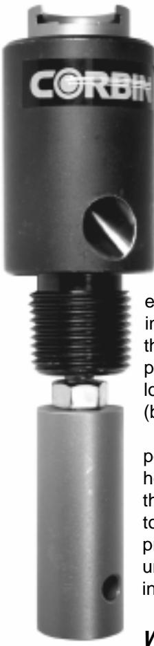
**A primer exhaust port** in the side of the adapter unit allows spent primers to drop free of the press ram. Stretching the split end of a piece of clear vinyl tubing (3/4 inch or larger) around the adapter will allow the spent primers to drop into the tubing and roll down it, into a waiting container.
