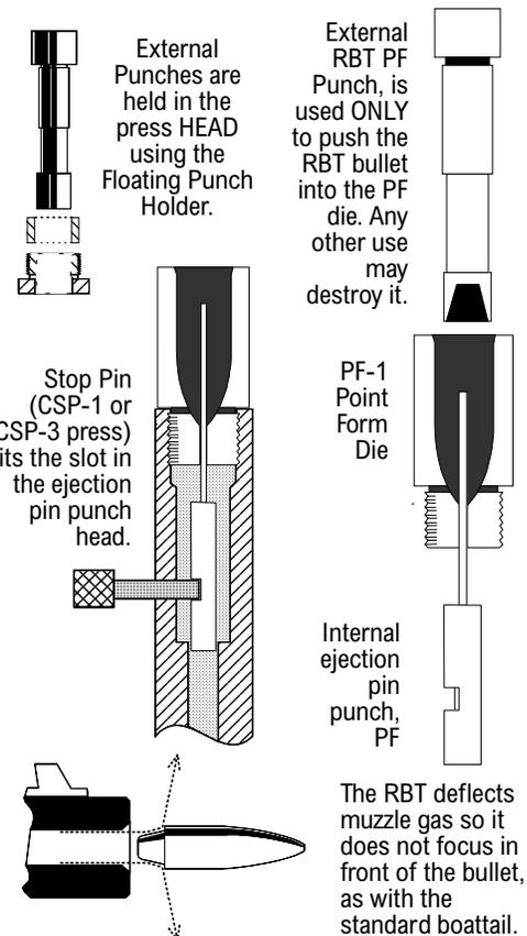
Never try to swage a component that will not go into the die by hand. The swaging operation depends on each component being slightly smaller than the die bore, and increases the bullet diameter a little with every step.
