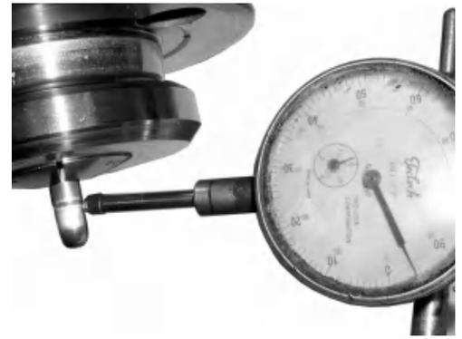
Holding the bullet in a precision collet and rotating it in a device with known, measurable run-out, such that a precision ground rod can be substituted for the bullet, and any run-out noted as the spindle is slowly turned can be marked at the high and low points with a marker pin on the front of the collet. This will let you know precisely how much and where the tool itself has consistent, repeatable run-out so you can subtract this from the bullet measurement.
