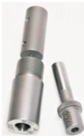
The core seating die is **CS-1-X**, and marked with a "**C**" for Core seat. It's purpose is to seat the lead core into the jacket.
