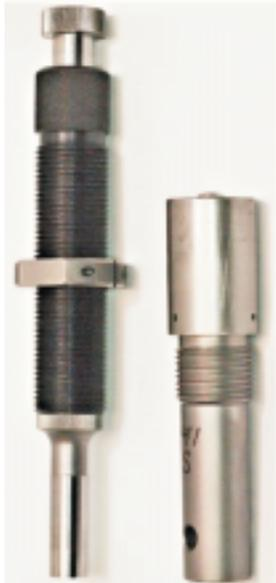
The **FPH-1-X** punch holder has a threaded draw bar. The end of the draw bar screws into the head of the top or external punch. Changing punches is done by turning the knob at the top to unscrew and free the punch. Corbin builds high quality 7/8-14 punch holders with steel split lock rings having wrench flats and hex socket locking screws. The punch holders are black oxide finished. Complete FPH-1-X, \$149.
